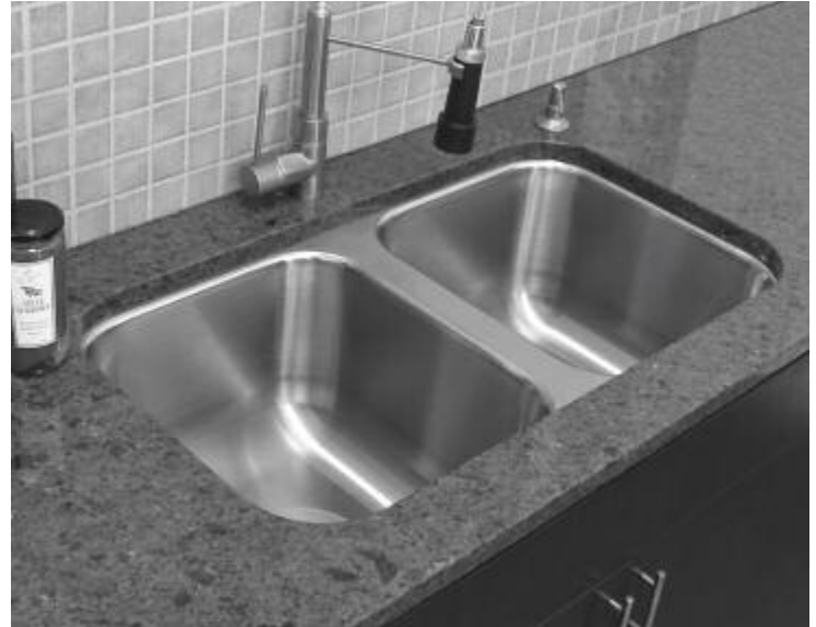
(There is a 1-1/4" flange on all 4 sides. We suggest leaving 3" clear in rear for rear mount faucet or faucet can also be mounted on side. Middle partition is 2-1/2" wide.) Faucet Not Included
